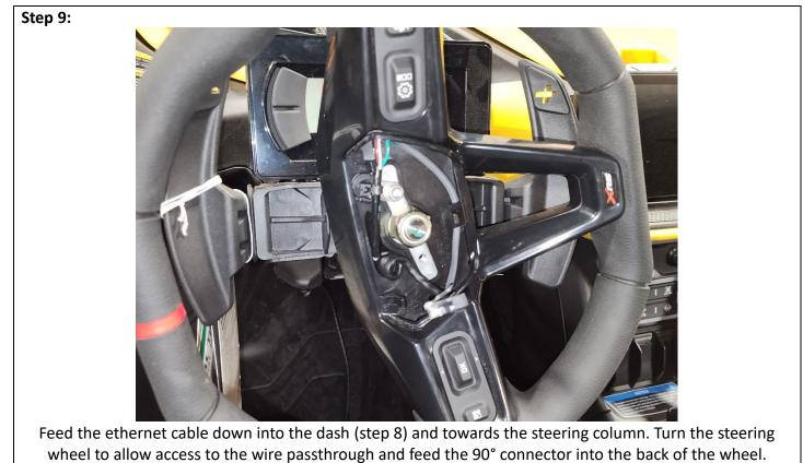
Ensure 2 full coils have been fed into the steering wheel.
